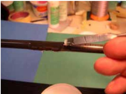
Then use the spatula to “level” the furrows and distribute it. To get an even edge of epoxy around the ends of the coated area use the “tire” technique described above.
