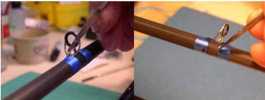
As the fishing rod is rotated form a bead of epoxy against the thread edge. With practice a thin or thick bead can be made in this way.
