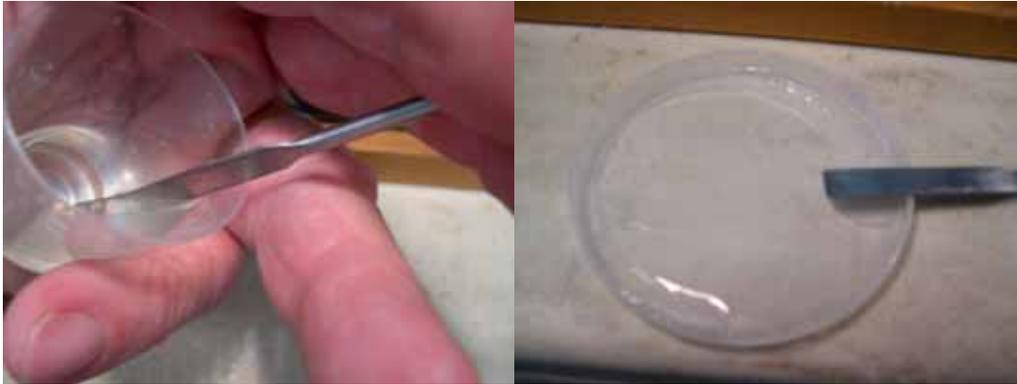
**Mix the hardener and resin together using the paddle end of the spatula. Use a slow mixing motion holding the spatula edge against the mixing cup edge. Periodically folding the mixture. Go slow so that excessive bubbles are not formed. Pour it out onto a flat surface after though mixing let it rest. This will reduce the thermal mass increasing pot life and allow bubbles to escape.**
