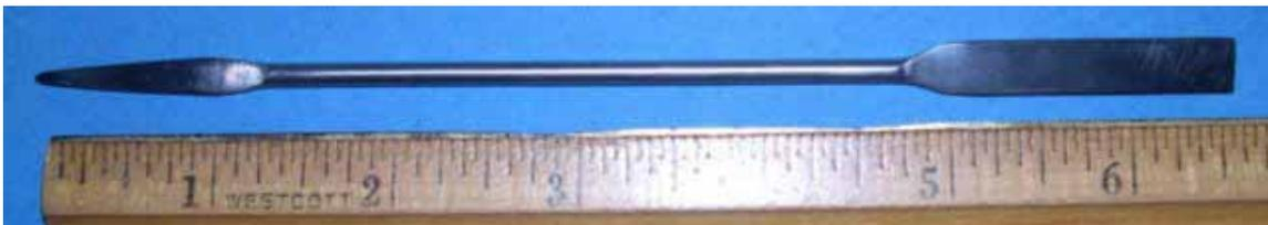
The pointed end is ground to a radius of approximately .030 inches. The finish is buffed and polished to a near mirror finish. Edges are ground and smoothed to a dull knife finish. This Fishing Rod Building tool is used to apply and mix epoxy finishes.
