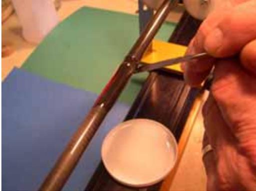
Many rod builders that cover thread weave designs apply epoxy along the fishing rod axis instead of around the circumference.
