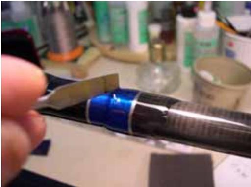
Holding the spatula perpendicular to the rod, place the edge of the blade end into the rotating epoxy. Only light pressure is needed here as the blade's edge could affect whatever the epoxy is covering if it is pressed onto the fishing rod with much pressure. A few examples of sensitive areas are inscriptions, decals, and feathers. Some inscriptions written with gel pens can be smeared quite easily.
