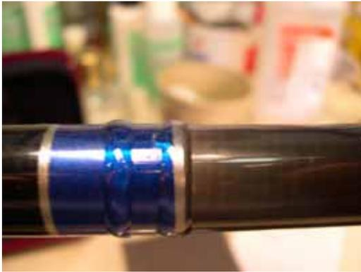
This tire bead will make an even finish edge around the circumference of the fishing rod. The epoxy will flow in and fill up against the tire as it turns. If there is insufficient epoxy add more. Repeat this step for the entire rod.
