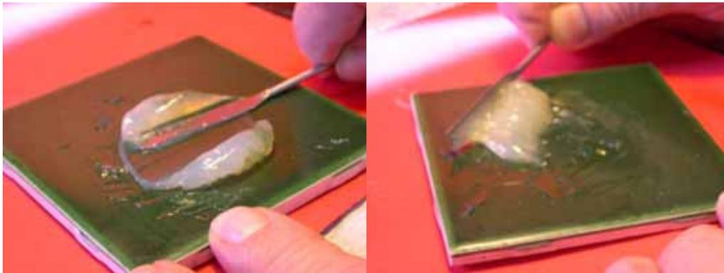
Use the paddle end for mixing by spreading and folding the resin and hardener together on the palette. Scrap the mixture off the palette surface using the edge of the spatula and fold it into itself to mix some more. The paste is fully mixed when the color becomes uniform throughout. The epoxy mixture will become slightly less thick as it is mixed. And you will notice how it acts as a lubricant as you scrape the palette.
